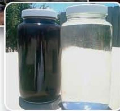
*Untreated reserve pit water (on left), and reclaimed water using the Green Machine*
